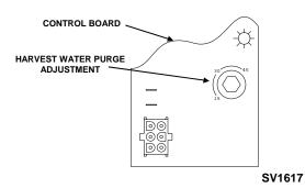
NOTE: The water purge **must be at the factory setting** of 45 seconds for the water inlet valve to energize during the last 15 seconds of the Water Purge. If set at 15 or 30 seconds the water inlet valve will not energize during the harvest water purge.
